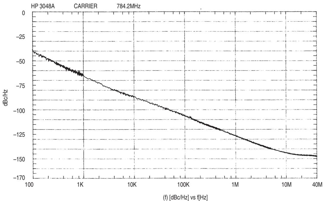
Figure 13. Typical Phase Noise Plot, 1200 MHz Tank
